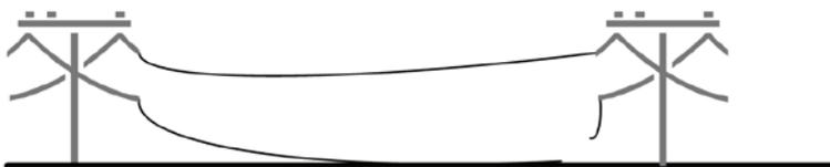
Figure 2: Downed Broken Conductor
