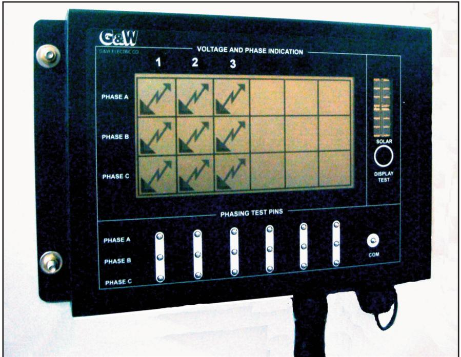
▲ Voltage Panel showing LCD display, display test button, solar panel and phasing test pins.
