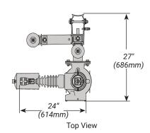
Polemount Bracket for Horizontal Insulator Configuration (15kV drawing shown)\*
