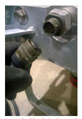
A standard hardwired control cable is provided on the Viper-SP module end. As an option, a connectorized module can be provided.
