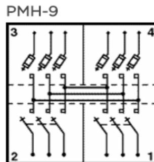
**Figure 3 – Air insulated Switchgear 9 Configuration**
