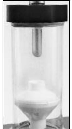
**B.** As the contacts separate, the SF<sub>6</sub> is compressed by the piston assembly and directed into the arc zone by the nozzle. The compressed SF<sub>6</sub> flows (is puffed) across the contacts and around the arc established by the separating puffed contacts. The cooling action of the gas is increased by the higher pressure (due to compression) and the flow which constantly provides a supply of cool SF<sub>6</sub> into the arc zone.
