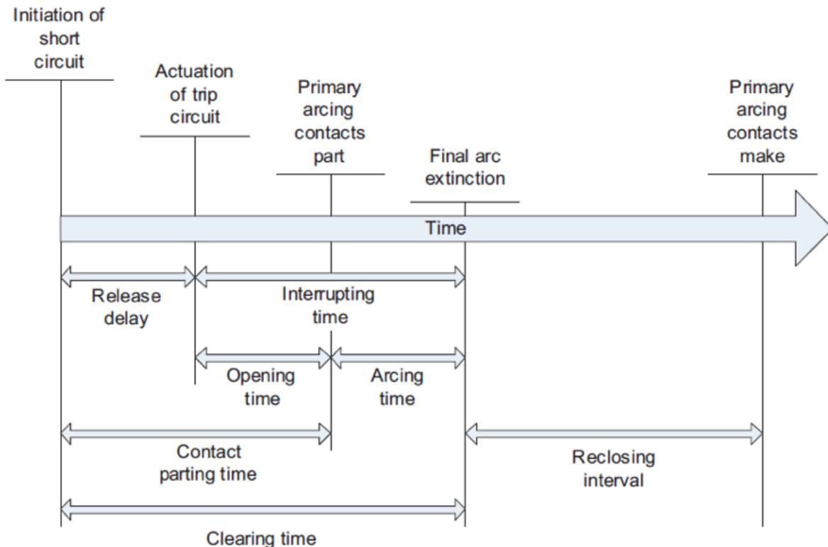
Figure 1: Graphical representation of Clearing Time
